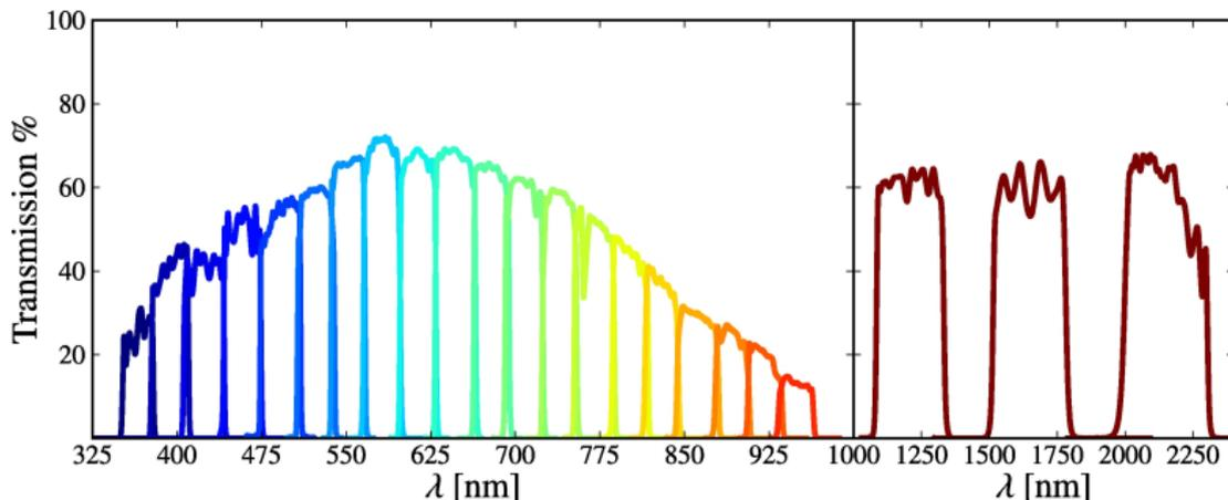
20 contiguous, non-overlapping medium-band ( $\sim 30$  nm) filters in the optical + 3 near-infrared filters ( $J$ ,  $H$ ,  $K_s$ ).
